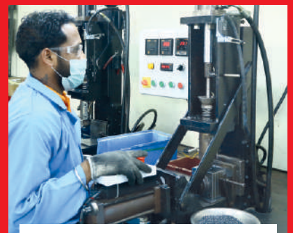
Semi - Automatic Moulding
